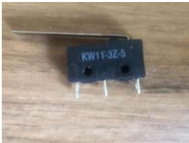
Fig. 24. Chaves Micro Switch KW11-3Z-5-3T.
