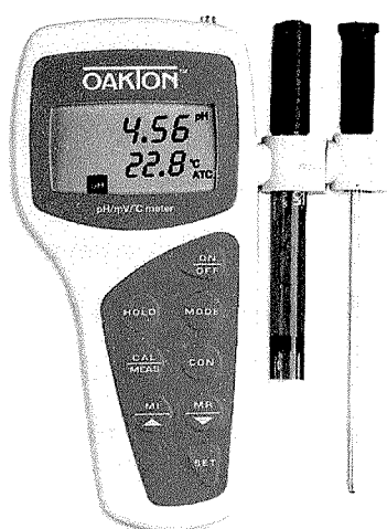
Fig. 10: pHmetro Oakton Modelo pH 100 Series
